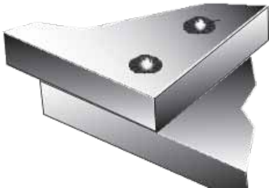
Plug Welds (Fig 1-19j)
