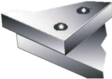
Plug Welds (Fig 1-19j)
